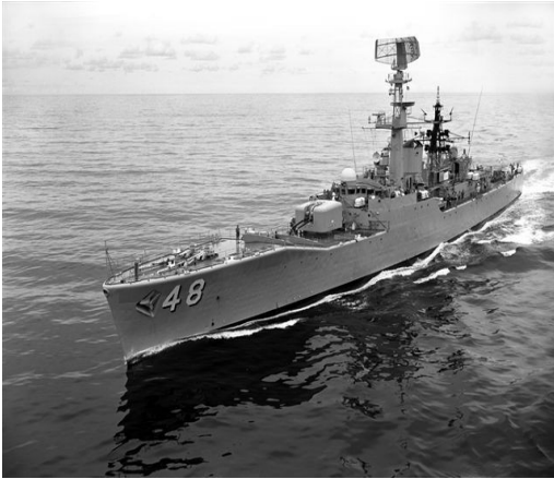
HMAS Stuart Prior to Modification in 1979 Note: Radar, Masts and Funnel Changes
